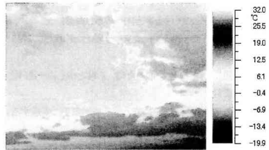
Fig-3 A sample image of the noise reduction : A result of the 8-neighbourhood median operator was applied to Fig-2.
