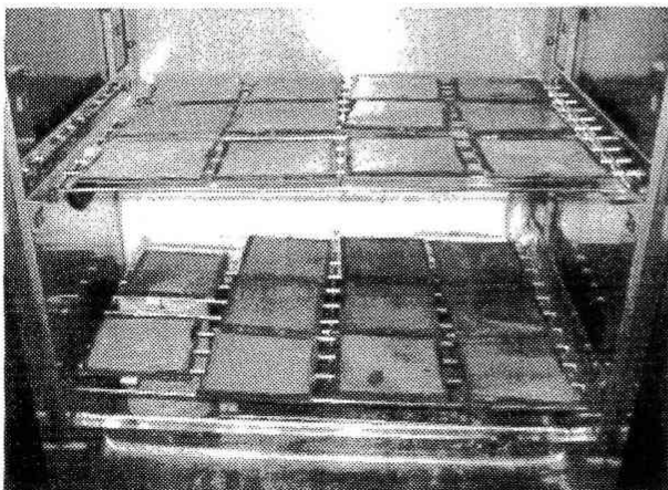
Fig. 9 Specimens of water vapor sorption test in temperature and humidity chamber
