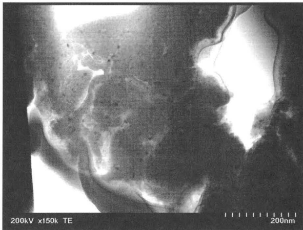
Fig. 9 STEM micrograph of \text{LaAl}_2\text{-V} mixture after 20 hours of mechanical alloying.
