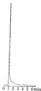
Fig. 2 Gas chromatogram of tri-iso-butylborane.
