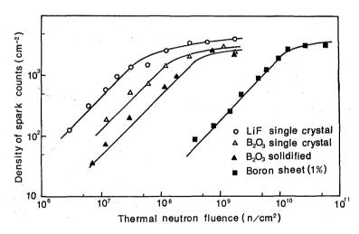
Fig. 2 Relation between thermal neutron fluence and density of spark counts
