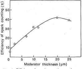
Fig. 3 Efficiecy of spark counting as function of moderator thickness
