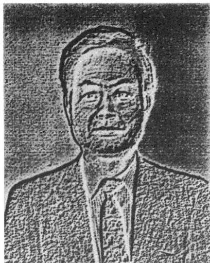
Fig.20 Experimental result of optical differentiation (Corresponding to \theta = 0 , \theta = \pi/2 and all direction)
