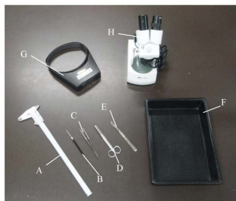
Fig. 2. Tools of anatomical experiment. A: vernier calipers, B: dissecting needle, C: tweezers, D: surgical scissors, E: knife, F: tray, G: binocular loupe, H: microscope.
