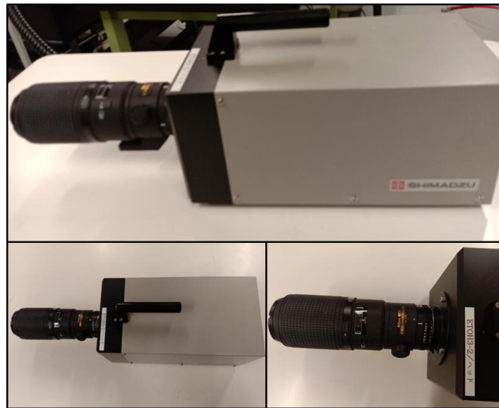
Figure 3.16 High-speed video camera Shimadzu mounted with a lens having a focal length of 20 cm
