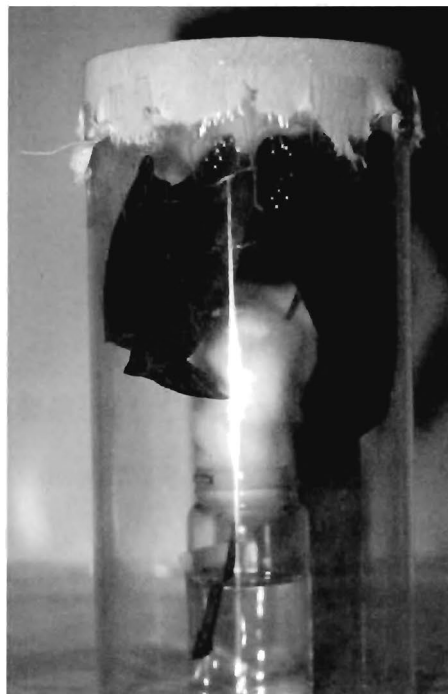
Fig. 5. Transparent plastic cylinder used in this study (20 cm high, 10 cm wide)
