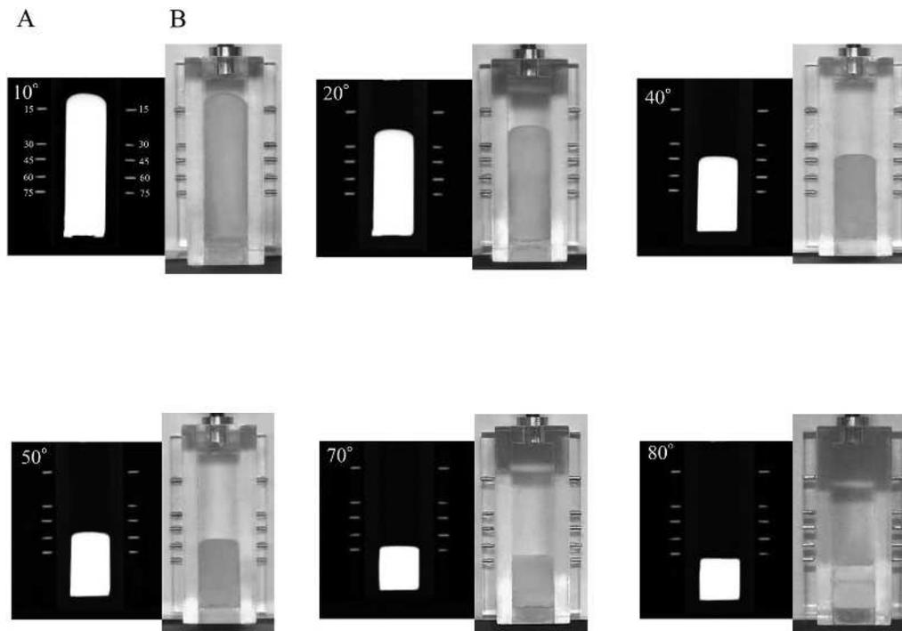
**Figure 6. Display ROT tilts of 10°, 20°, 40°, 50°, 70°, and 80° on X-ray images.** A, ROT on X-ray images. B, ROT indicating the respective scale. ROT: radiopaque tiltmeter.
