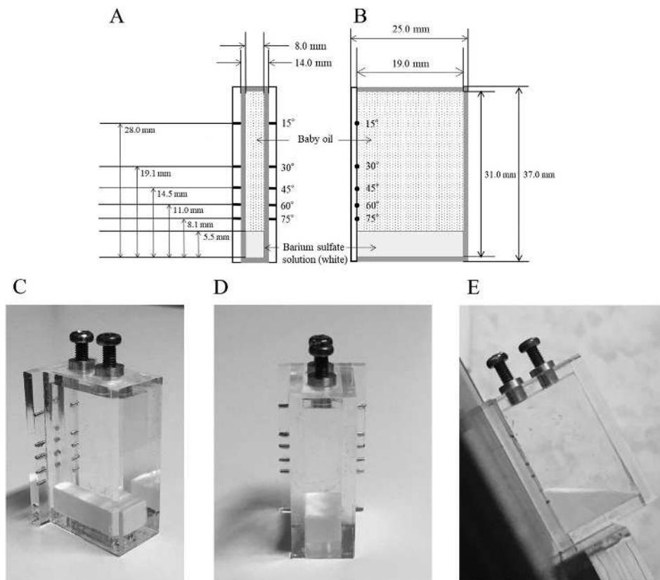
**Figure 1. Design of the ROT.** A, Schematic front-side view. B, Schematic right-side view. Based on a 2.0 mm polystyrene sheet, the internal dimensions were 8.0 mm (width) × 19.0 mm (length) × 31.0 mm (height). The heights at tilts of 15°, 30°, 45°, 60°, and 75° were 28.0, 19.1, 14.5, 11.0, and 8.1 mm, respectively. C, External view. D, Front-side view. E, Right-side view at a ROT tilt of 60°. The level of the radiopaque material indicates a tilt of 60°. ROT: radiopaque tiltmeter.
