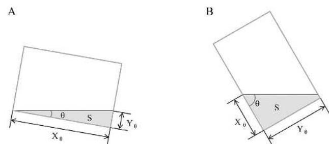
**Figure 2. Illustrations for calculations of the scale on the ROT.** A,  $\theta = 15^\circ, 30^\circ, 45^\circ$ . B,  $\theta = 60^\circ, 75^\circ$ .  $X_\theta$  and  $Y_\theta$  are the lengths of each side for a tilt of  $\theta$ .  $S$  is the area of the white barium sulfate solution.
