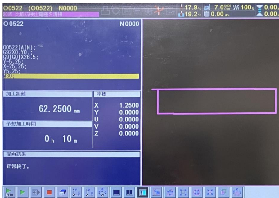
Fig. 11 The program that is being used to cut both of Ti-64 and TNTZ plate.
