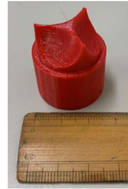
Fig. 4 Mold of valve membrane for vacuum forming.
