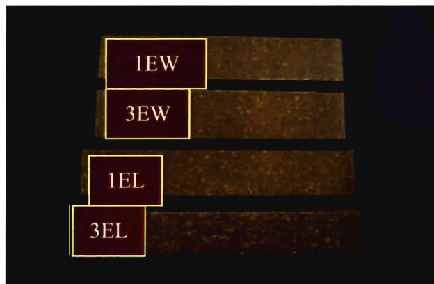
Figure 2.5. Standard cutting specimens of of extrusion molding composites. EL , Lengthwise (Dimensions: 0.92 \times 2.5 \times 10.8\text{cm} ); EW , Widthwise (Dimensions: 0.9 \times 1.9 \times 11.9\text{cm} )
