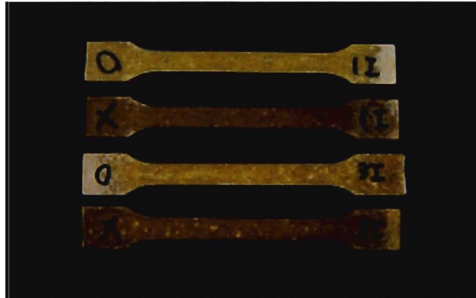
Figure 2.6. Dumbbell-shaped molds from injection molding method
