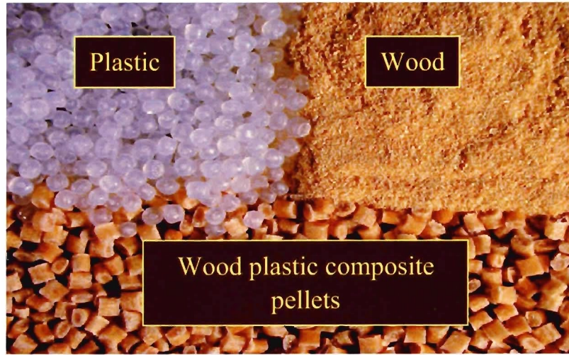
Figure 1.6. Pellets after processing of wood plastic composites
