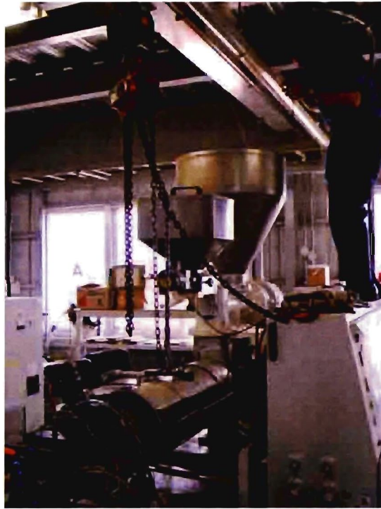
Figure 2.4. Conical twin-screw extruder model Titan 68
