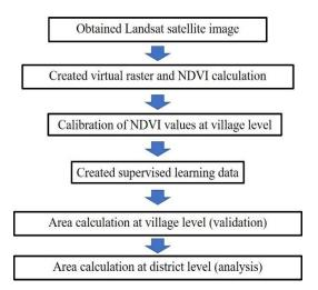
Fig. 2 Schematic flow of classification analysis using satellite data
