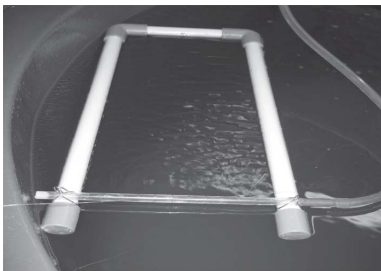
Fig. 3.1.2. The handcrafted surface skimmer which consisted of a rectangular floating trap and an air blower used in Experiment 1 and 2.
