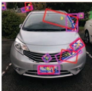
Fig. 14. License plate was not detected on a gray vehicle when same processing was performed with allowable brightness range left at 5.
