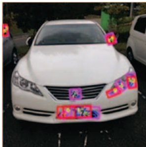
Fig. 13. License plate was detected in same vehicle when allowable brightness range was set to 5.
