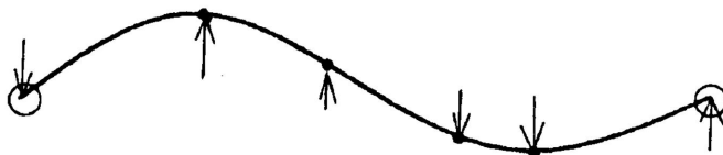
Fig. 1. Beam with unknown point load for interpolation
